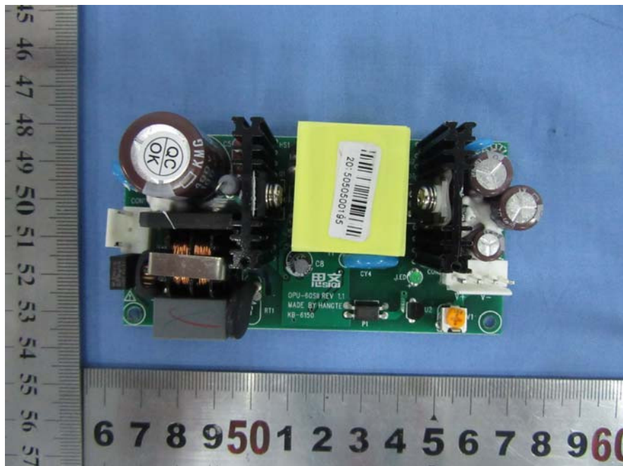
EUT – Power Board Top View
