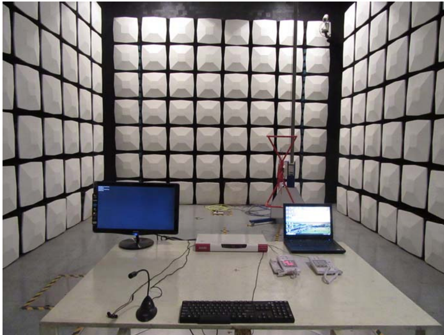
Radiated Emissions Test Setup - Front View (Below 1GHz)
