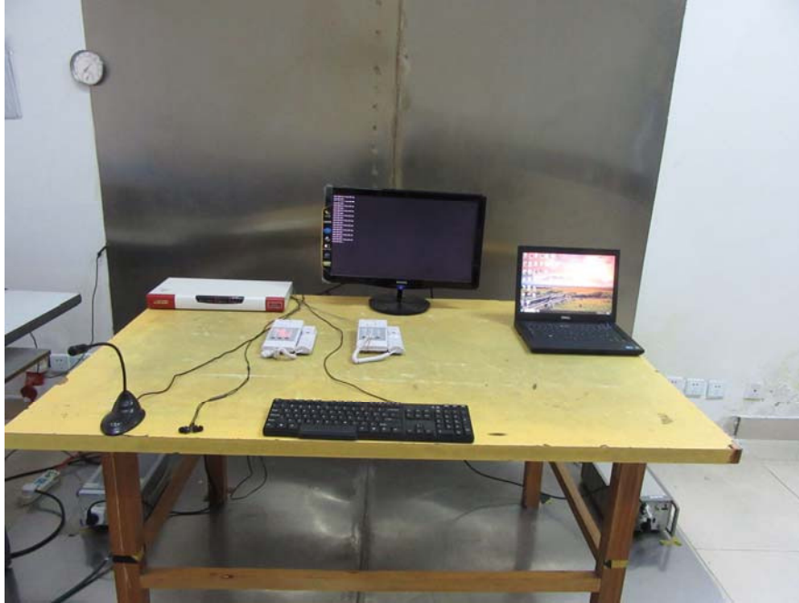
Conducted Emissions Test Setup – Front View
