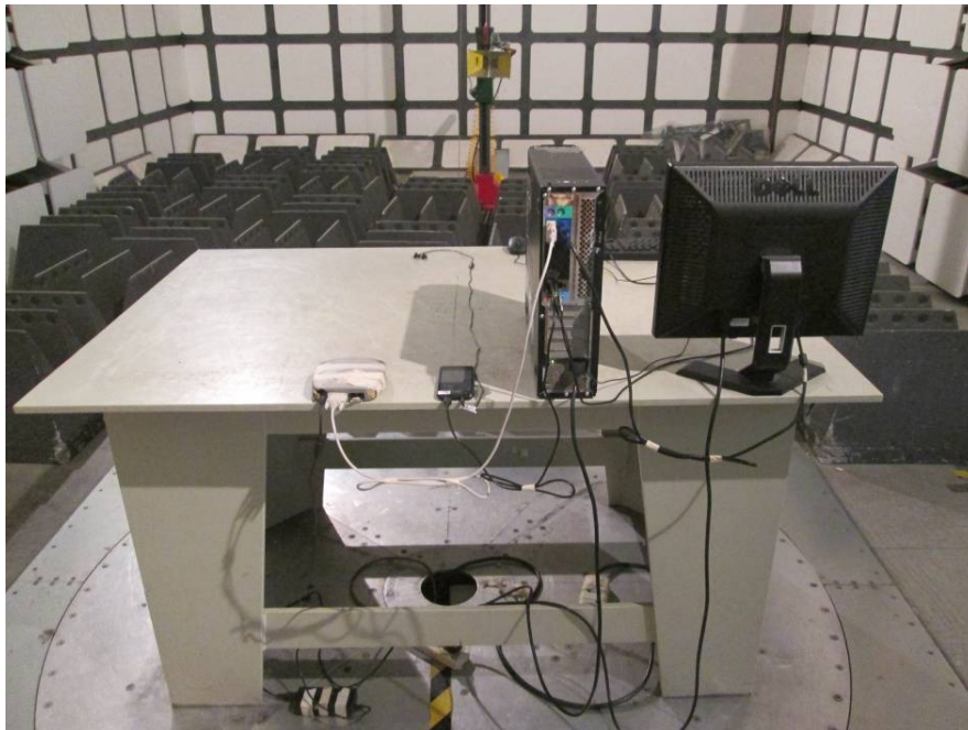
Radiated Emissions – Rear View (Above 1 GHz)
