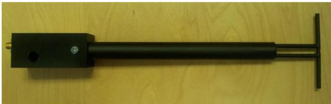
Figure 1 – MVG COMOSAR Validation Dipole
