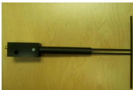
Figure 1 – MVG COMOSAR Validation Dipole
