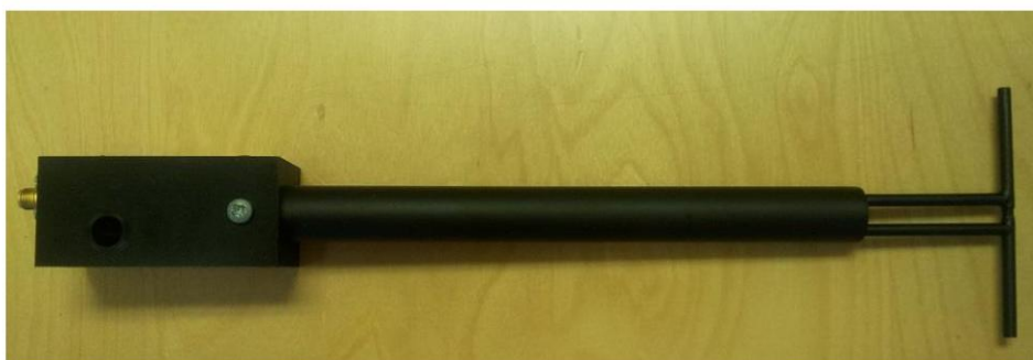
Figure 1 – MVG COMOSAR Validation Dipole
