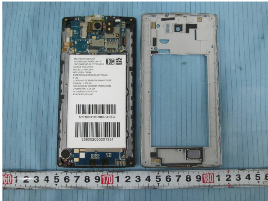
EUT –Cover off View 3
