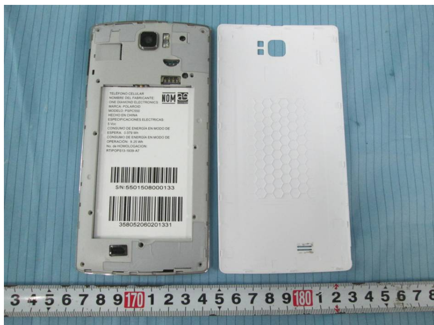
EUT –Cover off View 2
