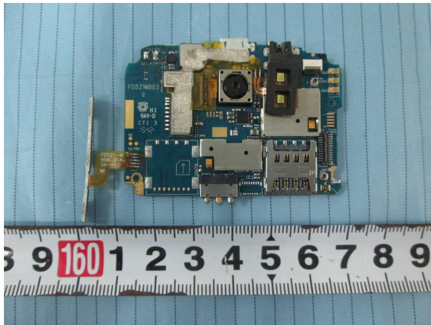
EUT – Main Board 1 Top View
