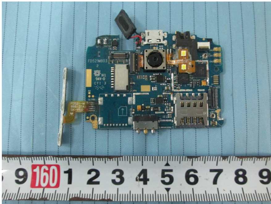
EUT – Main Board 1 Top Shielding off View
