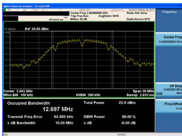
(802.11b) 6dB Bandwidth plot on channel 11
