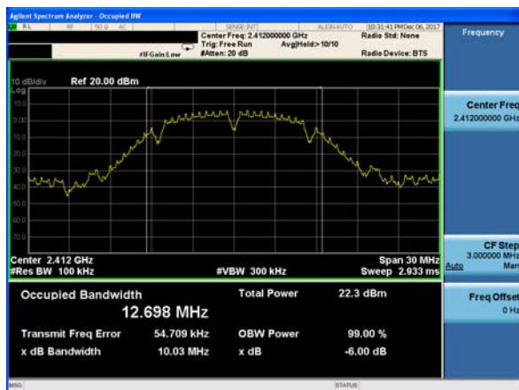
(802.11b) 6dB Bandwidth plot on channel 6
