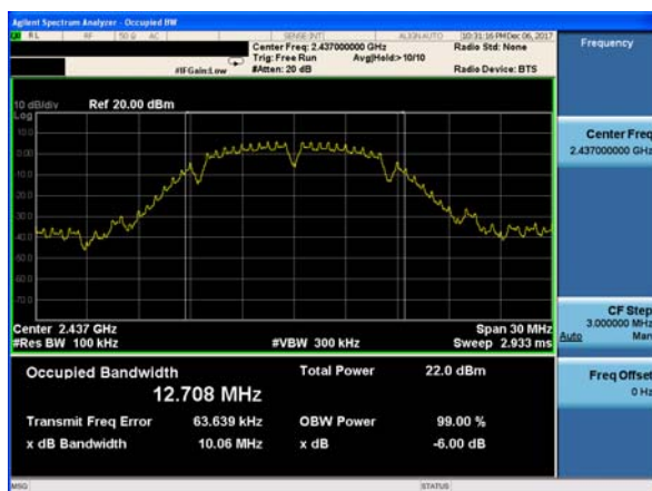
(802.11b) 6dB Bandwidth plot on channel 11
