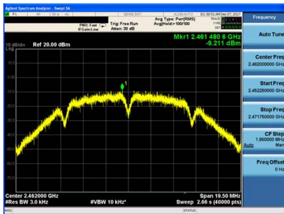
(802.11b) PSD plot on channel 11
