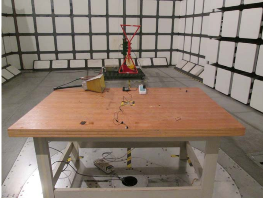
Radiated Emissions –Front View (30-1000 MHz)
