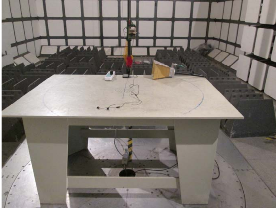
Radiated Emissions –Front View (1-25 GHz)
