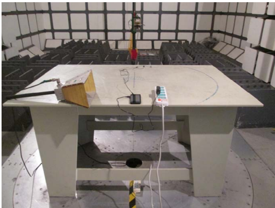
Radiated Emissions –Side View (1-25 GHz)
