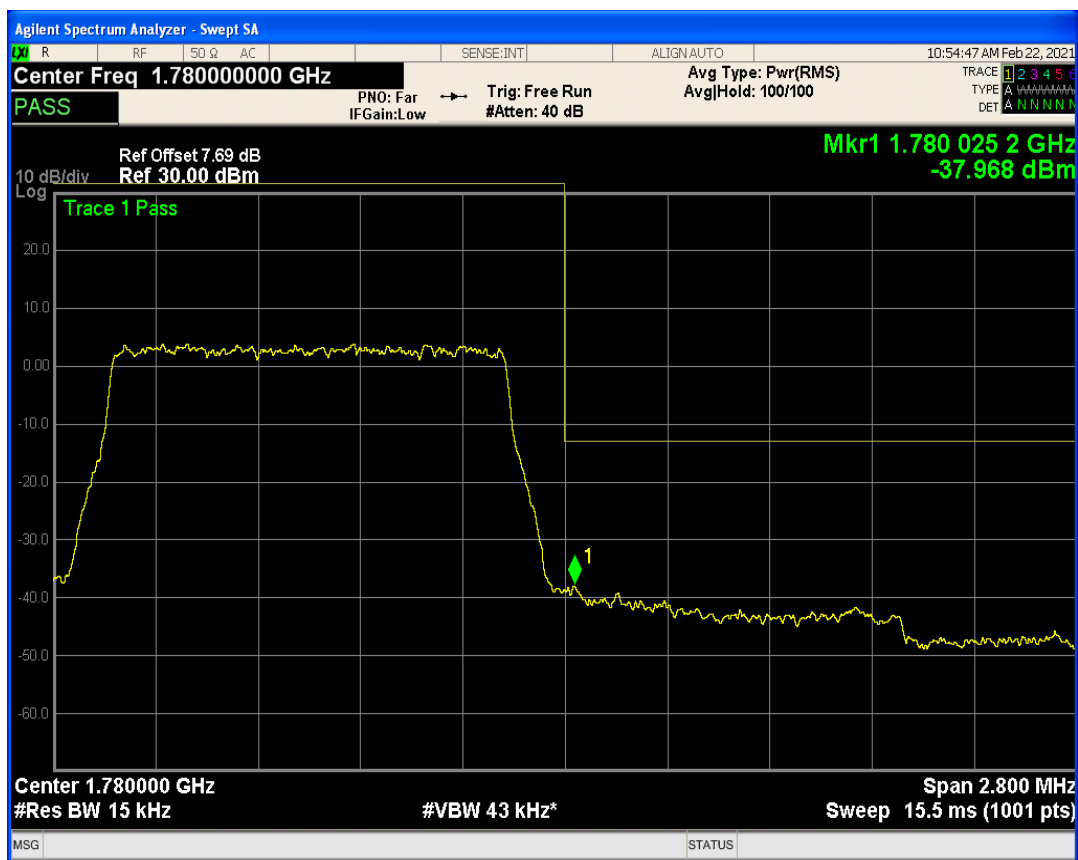
Band66 QPSK BW=10MHz Channel=132022 RB Size=1 Position=#0
