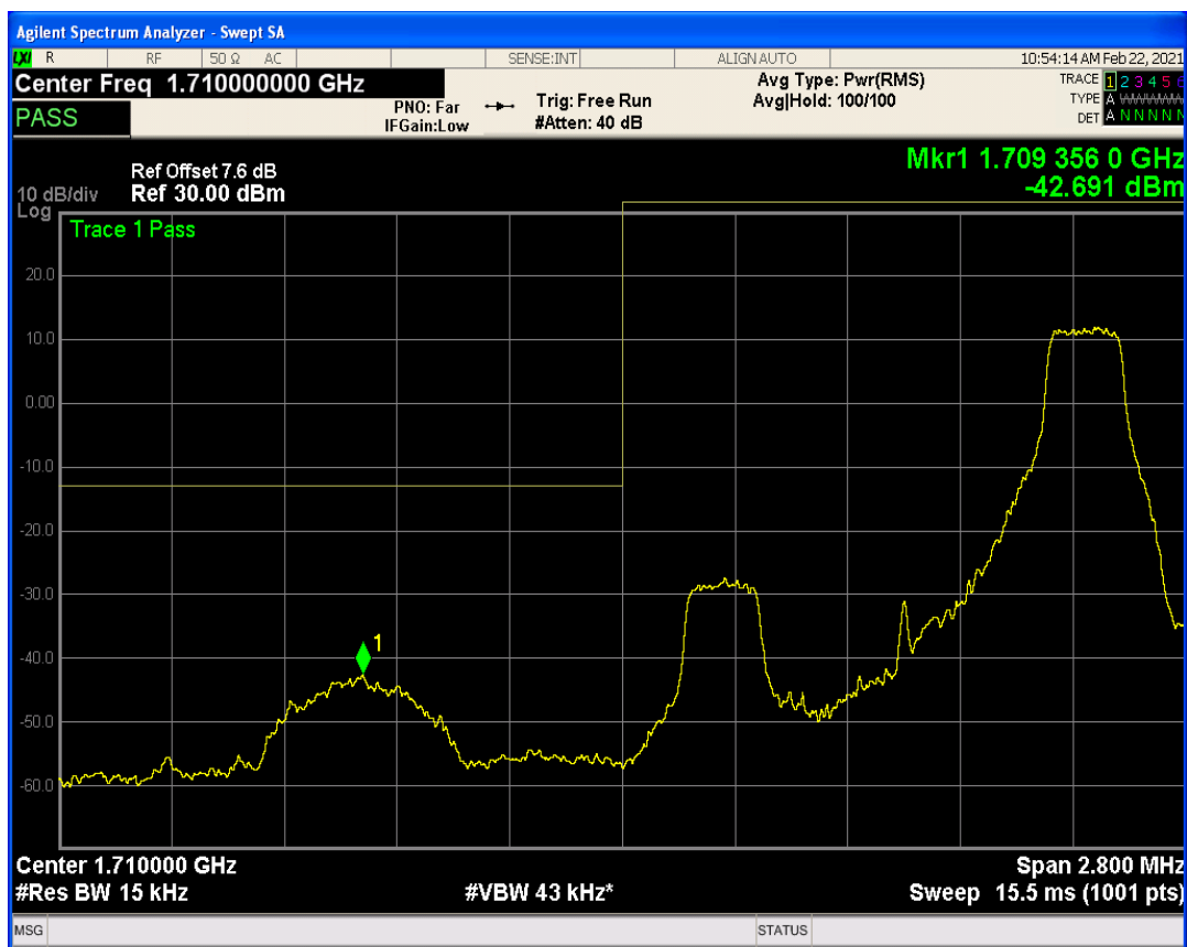
Band66 QAM16 BW=5MHz Channel=132647 RB Size=25 Position=#0
