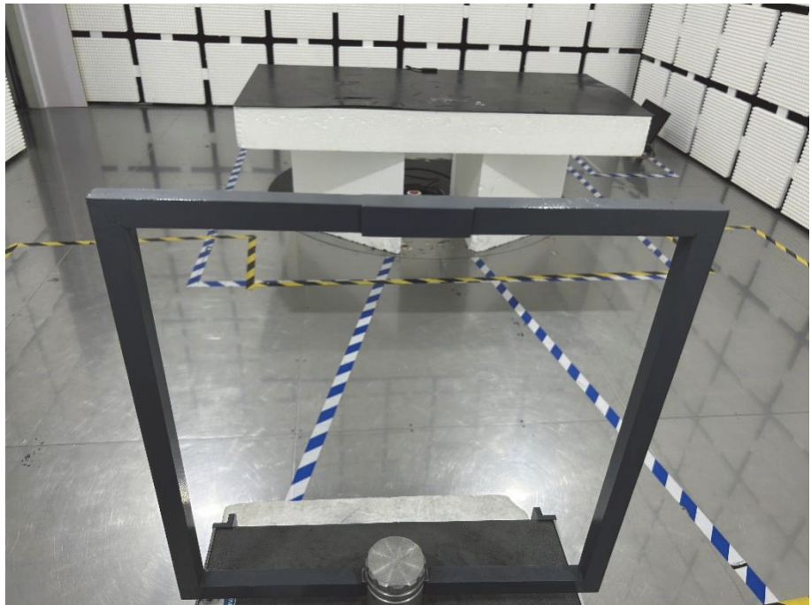
Radiation Emission Test Setup (Below 30MHz)
