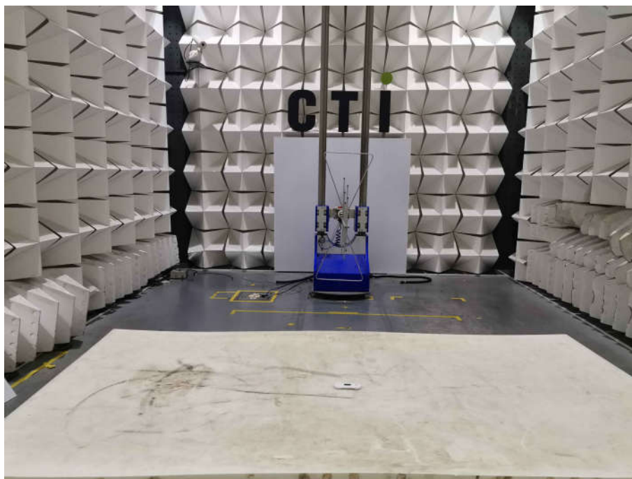
Radiated spurious emission Test Setup-1(Below 1GHz)
