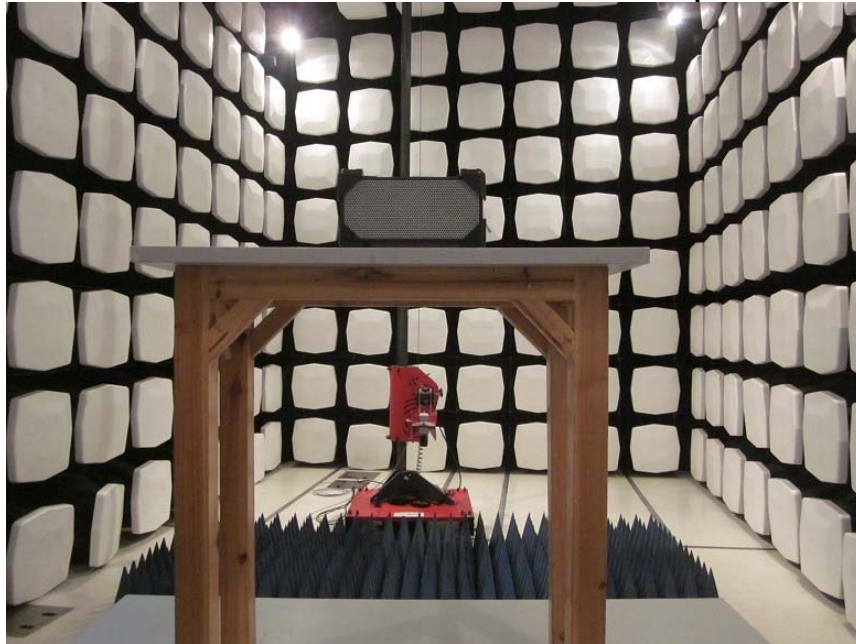
Measurement of Radiated Emission Test Set Up
