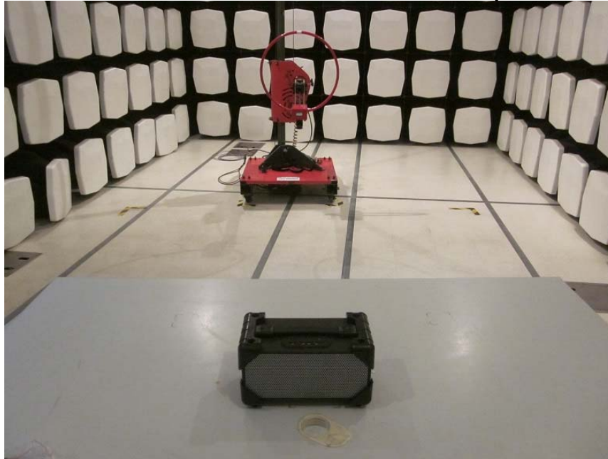
Measurement of Radiated Emission Test Set Up
