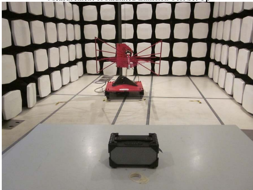
Measurement of Radiated Emission Test Set Up
