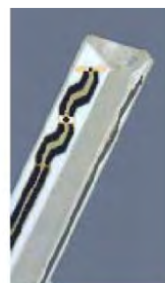
Figure E.2.2 Probe Thick-Film Technique
