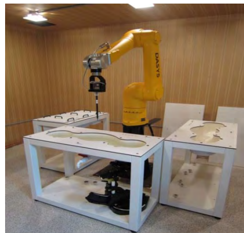
Figure E.7.1 DASY5 Test System
