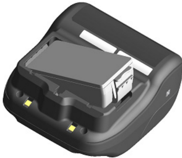
Figure 8-2 Installing Battery Pack (1)
