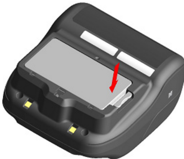
Figure 8-3 Installing Battery Pack (2)
