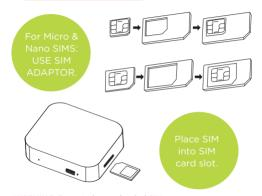
WARNING: Do not place unloaded SIM adaptor into the SmartBox as it may cause permanent damage to the SmartBox)
