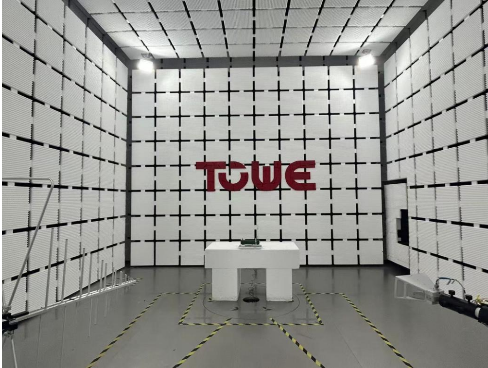
Radiated Emission Below 1GHz
