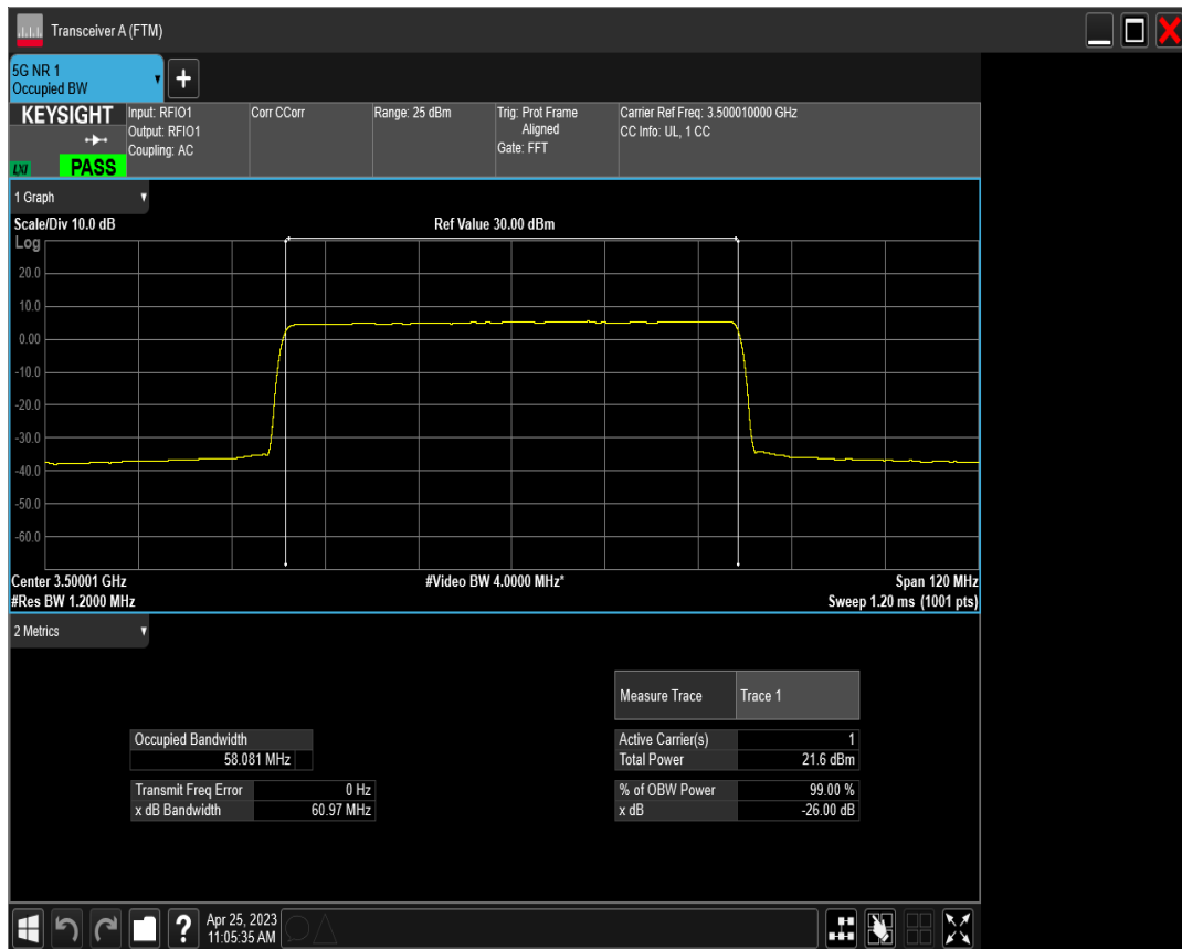
n77(3450-3550) SCS=30kHz CP_QPSK BW=60MHz Channel=633334 RB=162@0
