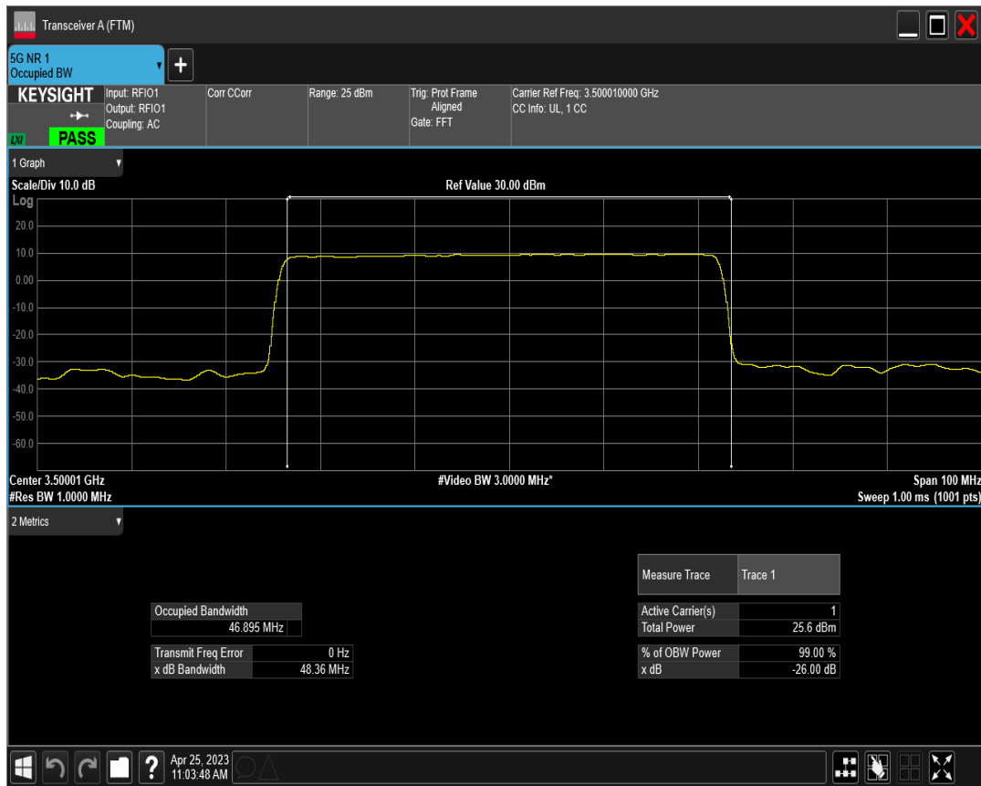
n77(3450-3550) SCS=30kHz DFT_QPSK BW=50MHz Channel=633334 RB=128@0
