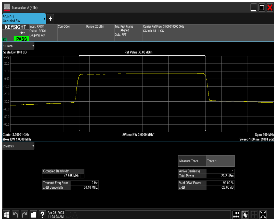
n77(3450-3550) SCS=30kHz DFT_BPSK BW=50MHz Channel=635000 RB=128@0
