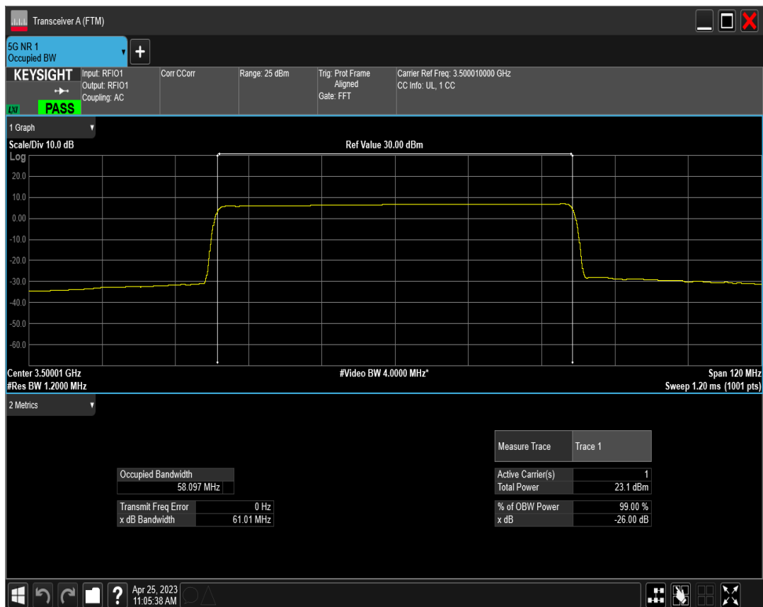
n77(3450-3550) SCS=30kHz DFT_BPSK BW=60MHz Channel=634666 RB=162@0
