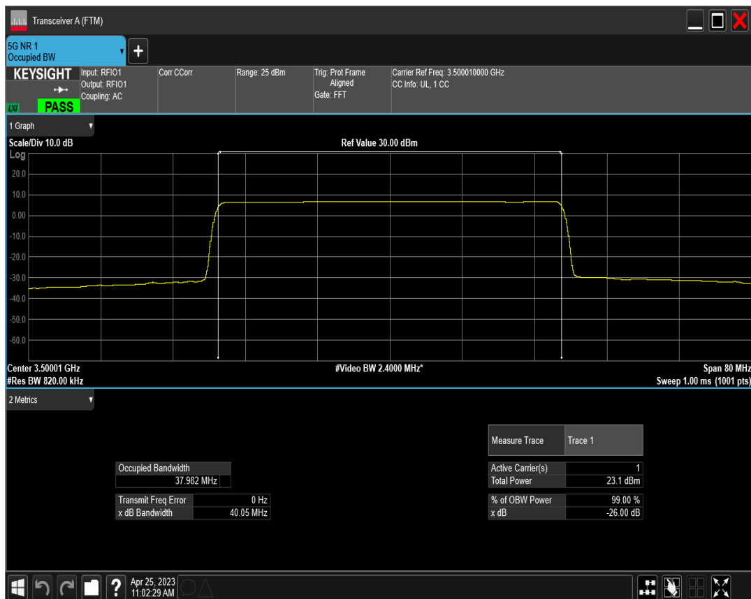
n77(3450-3550) SCS=30kHz DFT_BPSK BW=40MHz Channel=635332 RB=100@0
