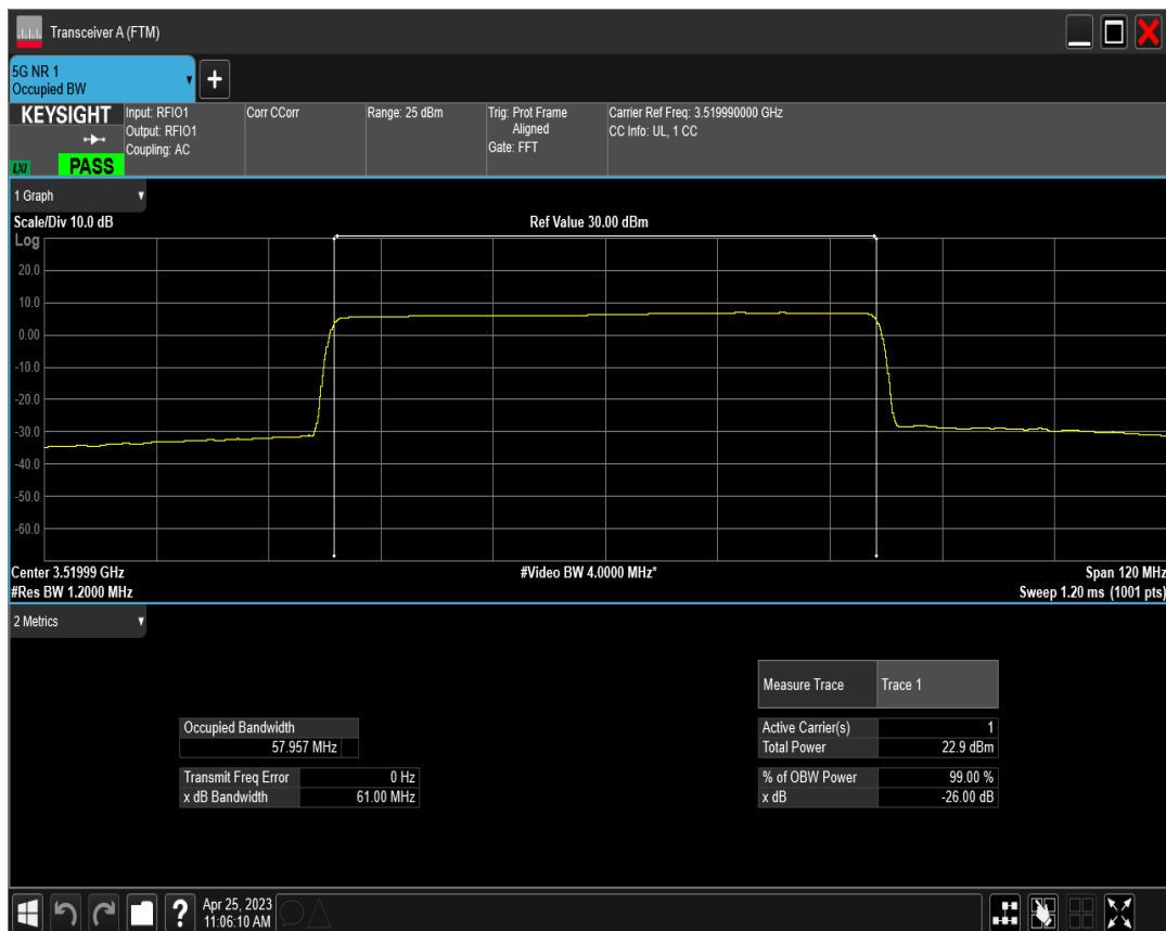
n77(3450-3550) SCS=30kHz DFT_BPSK BW=80MHz Channel=632668 RB=216@0
