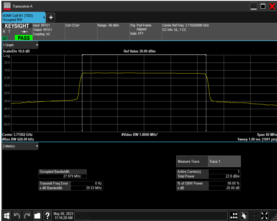
n77(3700-3980) SCS=30kHz DFT_BPSK BW=30MHz Channel=656000 RB=75@0
