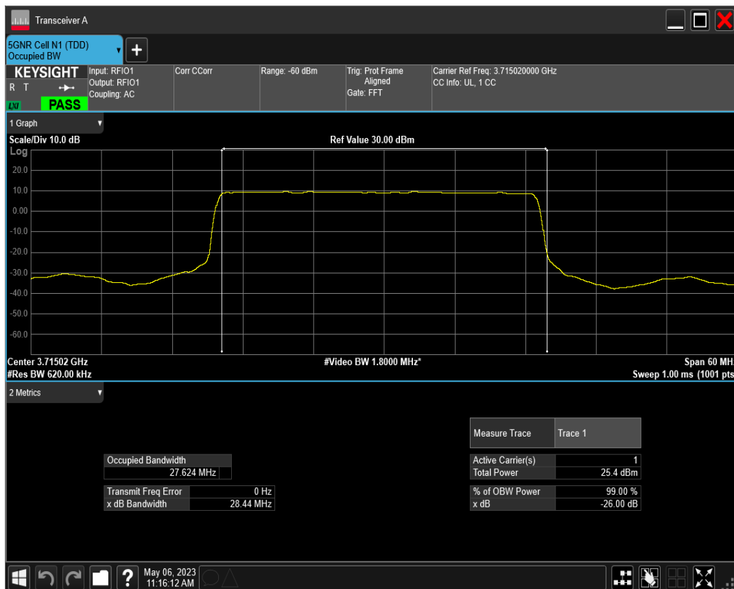
n77(3700-3980) SCS=30kHz DFT_QPSK BW=30MHz Channel=647668 RB=75@0
