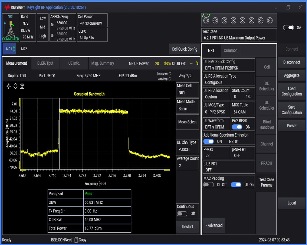
n78(3700-3800) SCS=30kHz DFT_BPSK BW=80MHz Channel=650000 RB=216@0
