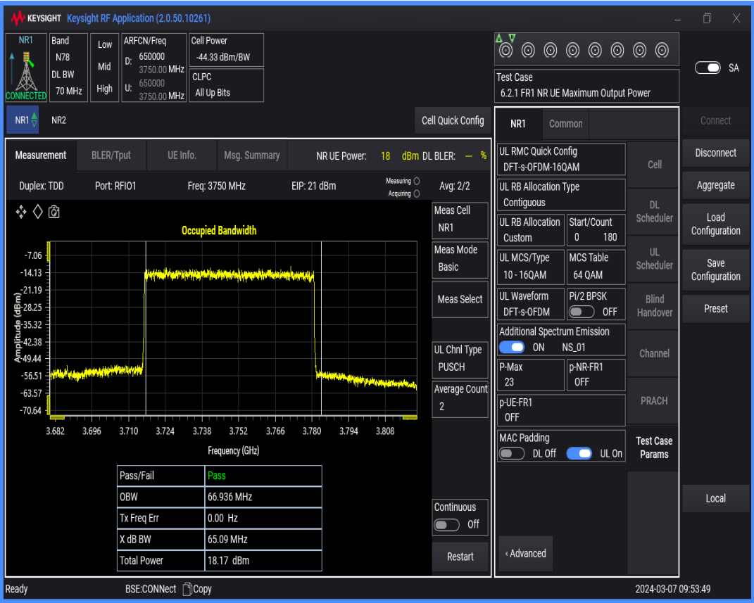
n78(3700-3800) SCS=30kHz DFT_QAM16 BW=80MHz Channel=650000 RB=216@0
