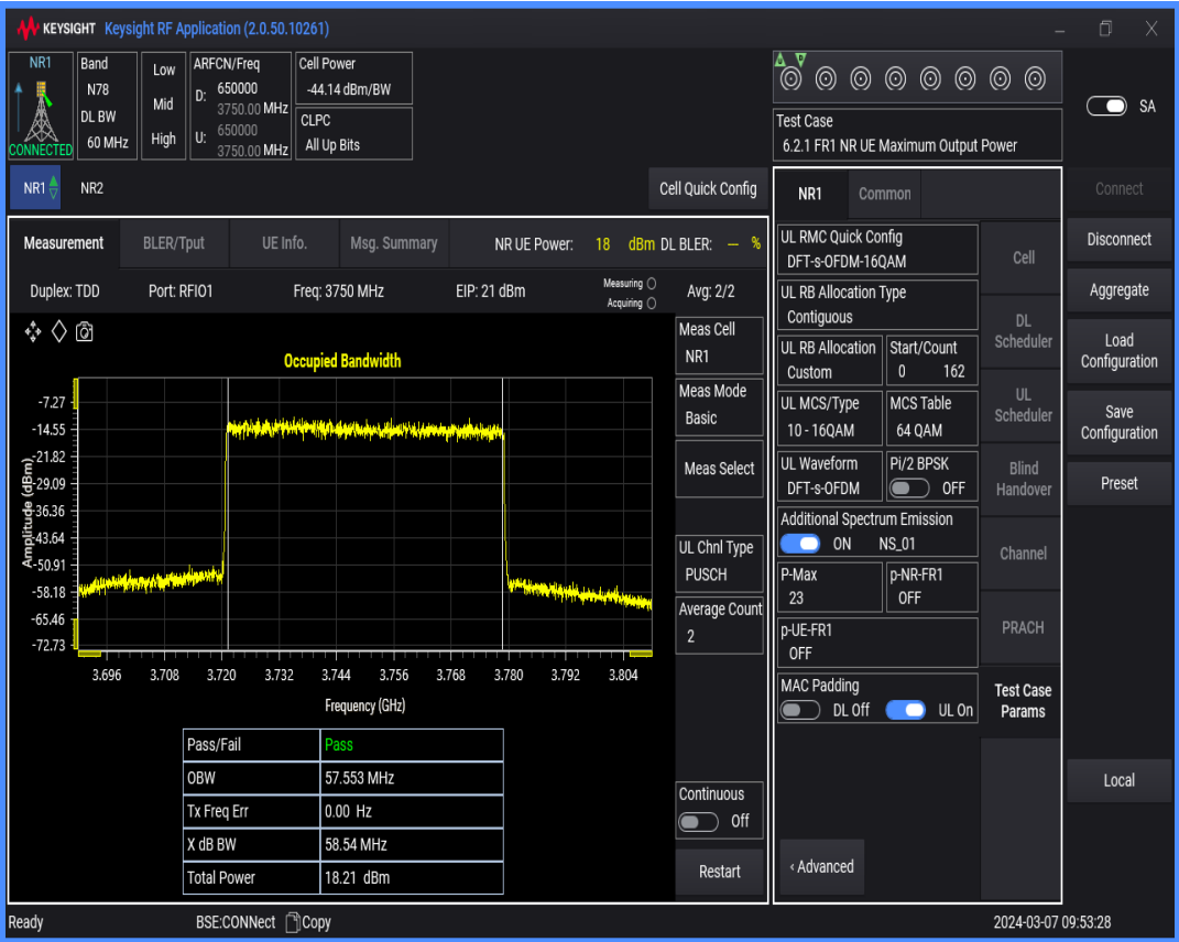
n78(3700-3800) SCS=30kHz DFT_QAM16 BW=70MHz Channel=650000 RB=
