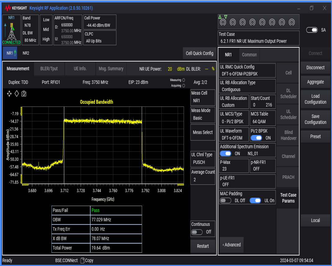
n78(3700-3800) SCS=30kHz DFT_BPSK BW=90MHz Channel=650000 RB=240@0
