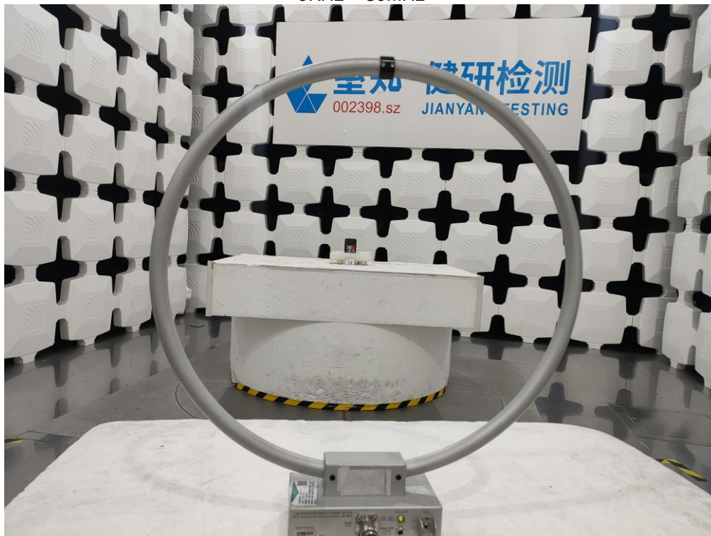
Radiated Spurious Emission 9KHz ~ 30MHz
