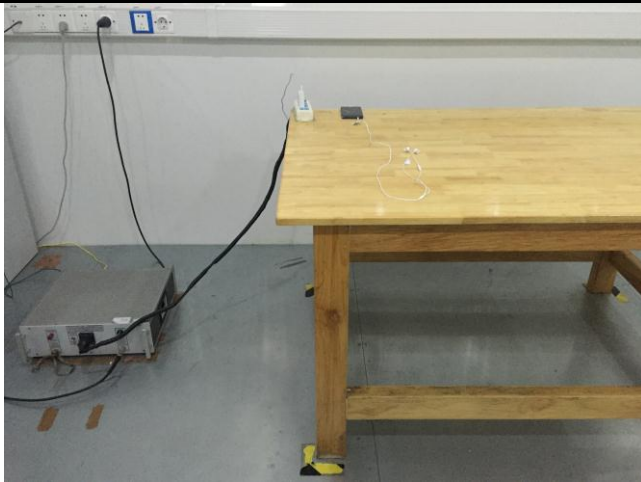
Conducted Emissions Test Setup Front View
