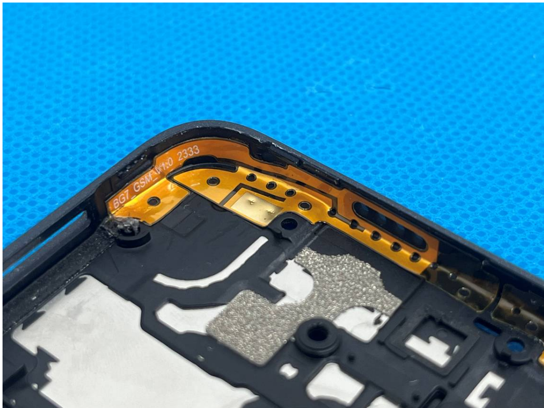
WWAN Main ANT (GSM850/WCDMA B5/LTE B5/12/17)
