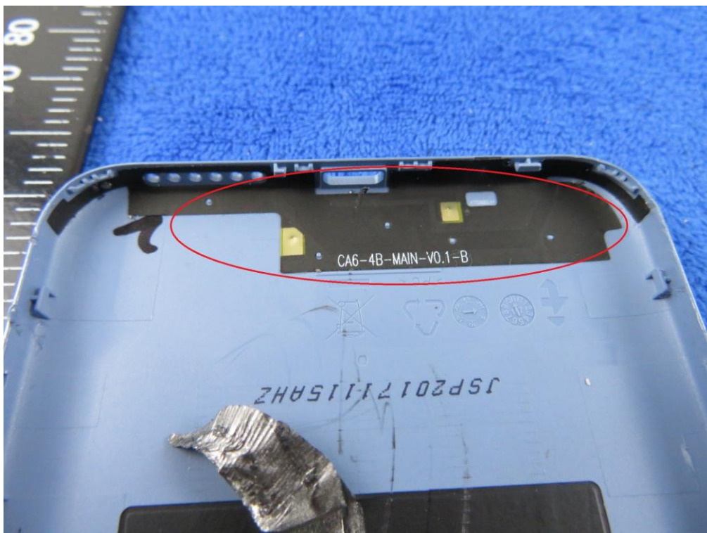
GSM/PCS/UMTS-FDD/LTE Antenna View
