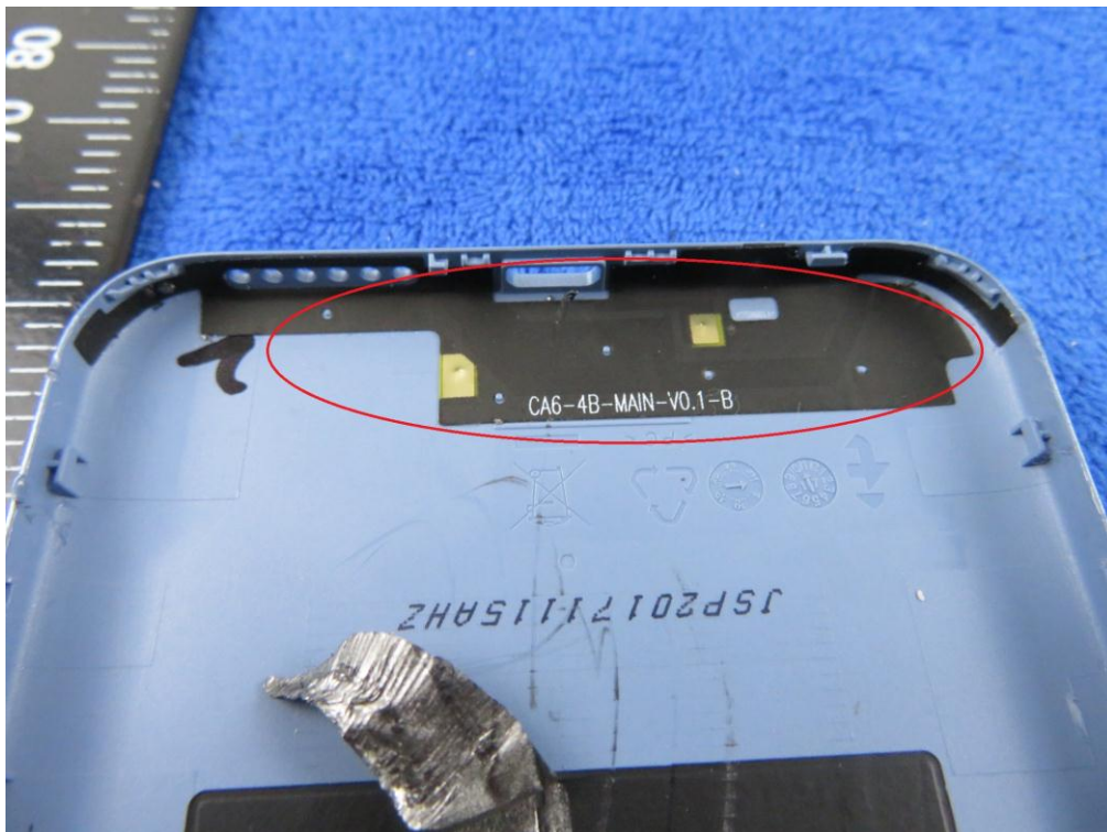
GSM/PCS/UMTS-FDD/LTE Antenna View
