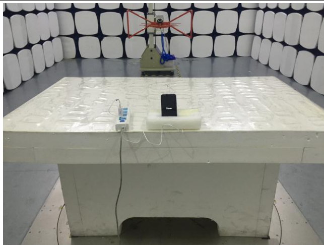
Conducted Emissions Test Setup Front View
