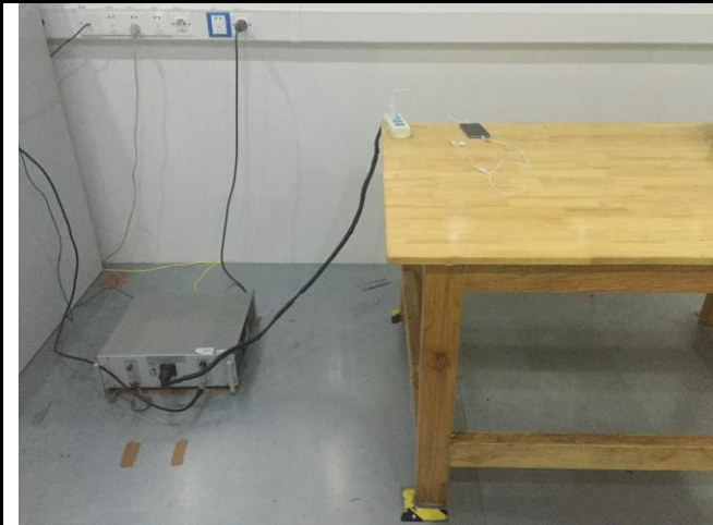
Conducted Emissions Test Setup Front View
