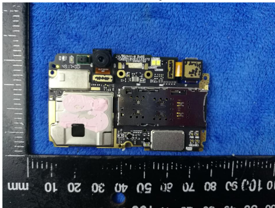
Mainboard with Shielding - Rear View
