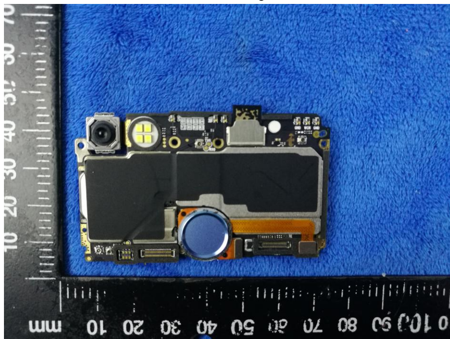
Mainboard with Shielding - Front View
