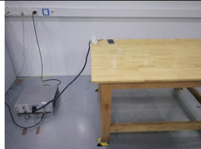
Conducted Emissions Test Setup Front View
