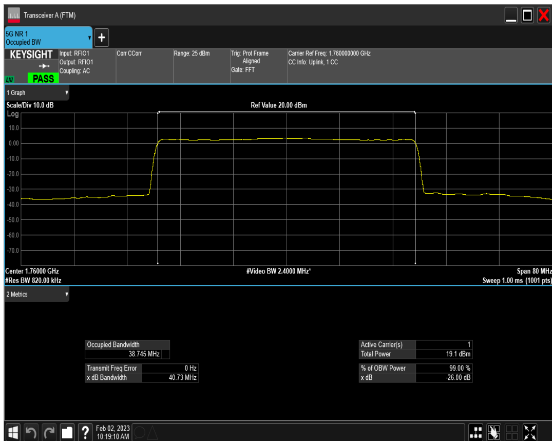
n66 SCS=15kHz DFT_QAM64 BW=40MHz Channel=352000 RB=216@0
