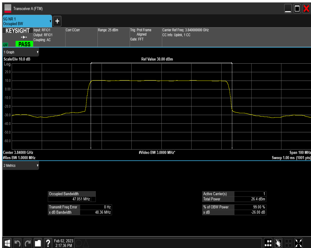
n77(3700-3980) SCS=30kHz DFT_QPSK BW=50MHz Channel=656000 RB=128@0
