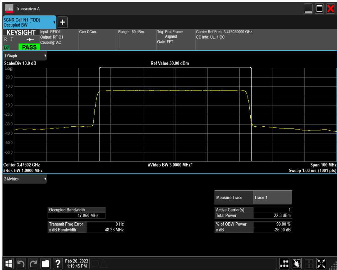
n77(3450-3550) SCS=30kHz CP_QPSK BW=50MHz Channel=631668 RB=133@0
