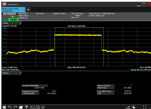
70MHz_30kHz_3500MHz_DFT-s-OFDM PI/2 BPSK_RB180@0 66.877 MHz
