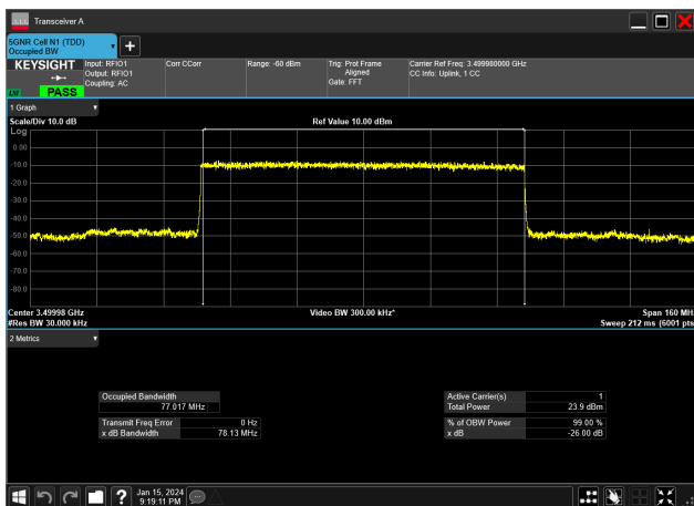
80MHz_30kHz_3500MHz_DFT-s-OFDM QPSK_RB216@0 77.017 MHz
