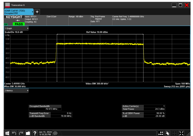
80MHz_30kHz_3500MHz_DFT-s-OFDM PI/2 BPSK_RB216@0 76.973 MHz
