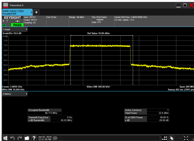
70MHz_30kHz_3485MHz_DFT-s-OFDM 64 QAM_RB180@0 66.713 MHz
