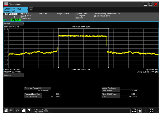
70MHz_30kHz_3515MHz_DFT-s-OFDM PI/2 BPSK_RB180@0 66.929 MHz
