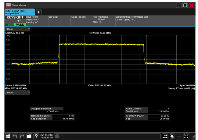
50MHz_30kHz_3500MHz_DFT-s-OFDM 16 QAM_RB128@0 47.065 MHz
