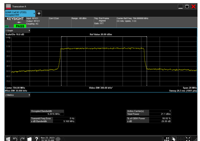
10MHz_15kHz_704MHz_DFT-s-OFDM 16 QAM_RB50@0 9.202 MHz
