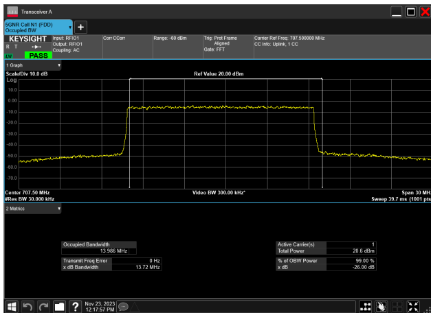
15MHz_15kHz_707.5MHz_DFT-s-OFDM 64 QAM_RB75@0 13.986 MHz
