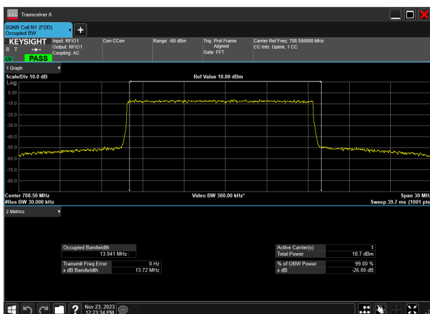
15MHz_15kHz_708.5MHz_DFT-s-OFDM 256 QAM_RB75@0 13.941 MHz
