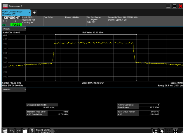
15MHz_15kHz_706.5MHz_DFT-s-OFDM 256 QAM_RB75@0 13.938 MHz
