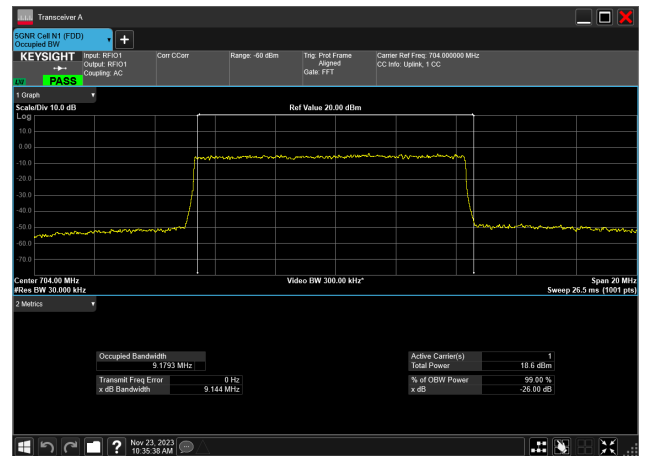
10MHz_15kHz_704MHz_DFT-s-OFDM 256 QAM_RB50@0 9.179 MHz
