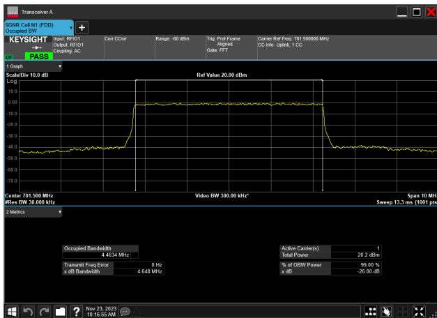
5MHz_15kHz_701.5MHz_CP-OFDM 16 QAM_RB25@0 4.463 MHz
