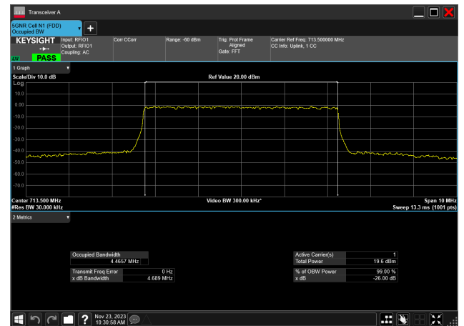
5MHz_15kHz_713.5MHz_CP-OFDM 64 QAM_RB25@0 4.466 MHz
