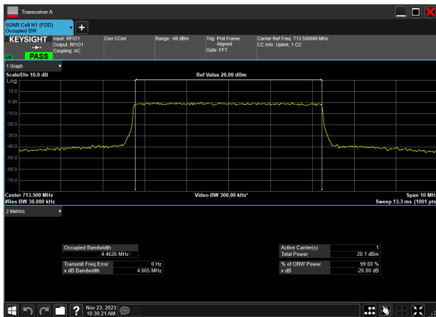
5MHz_15kHz_713.5MHz_CP-OFDM 16 QAM_RB25@0 4.463 MHz
