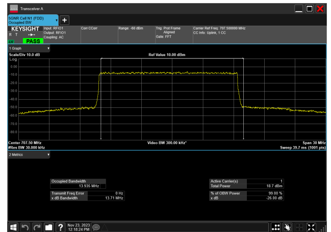
15MHz_15kHz_707.5MHz_DFT-s-OFDM 256 QAM_RB75@0 13.935 MHz
