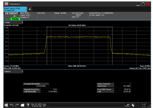
10MHz_15kHz_711MHz_DFT-s-OFDM 256 QAM_RB50@0 9.216 MHz
