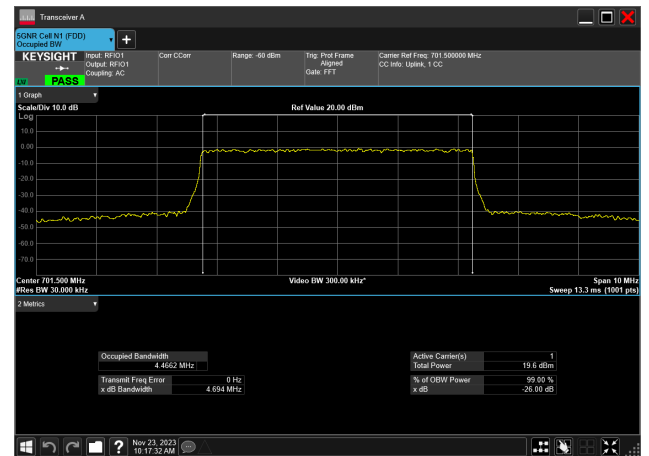
5MHz_15kHz_701.5MHz_CP-OFDM 64 QAM_RB25@0 4.466 MHz
