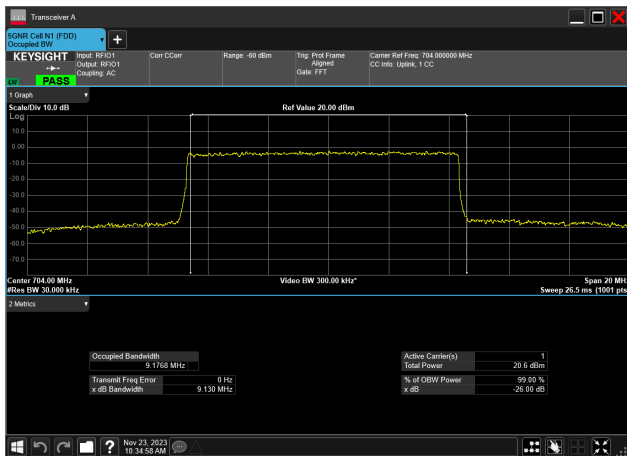
10MHz_15kHz_704MHz_DFT-s-OFDM 64 QAM_RB50@0 9.177 MHz
