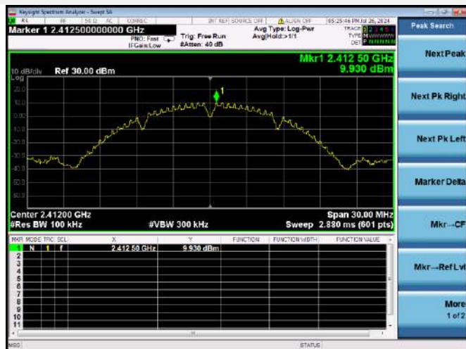
802.11b LOW CHANNEL, CARRIER LEVEL
