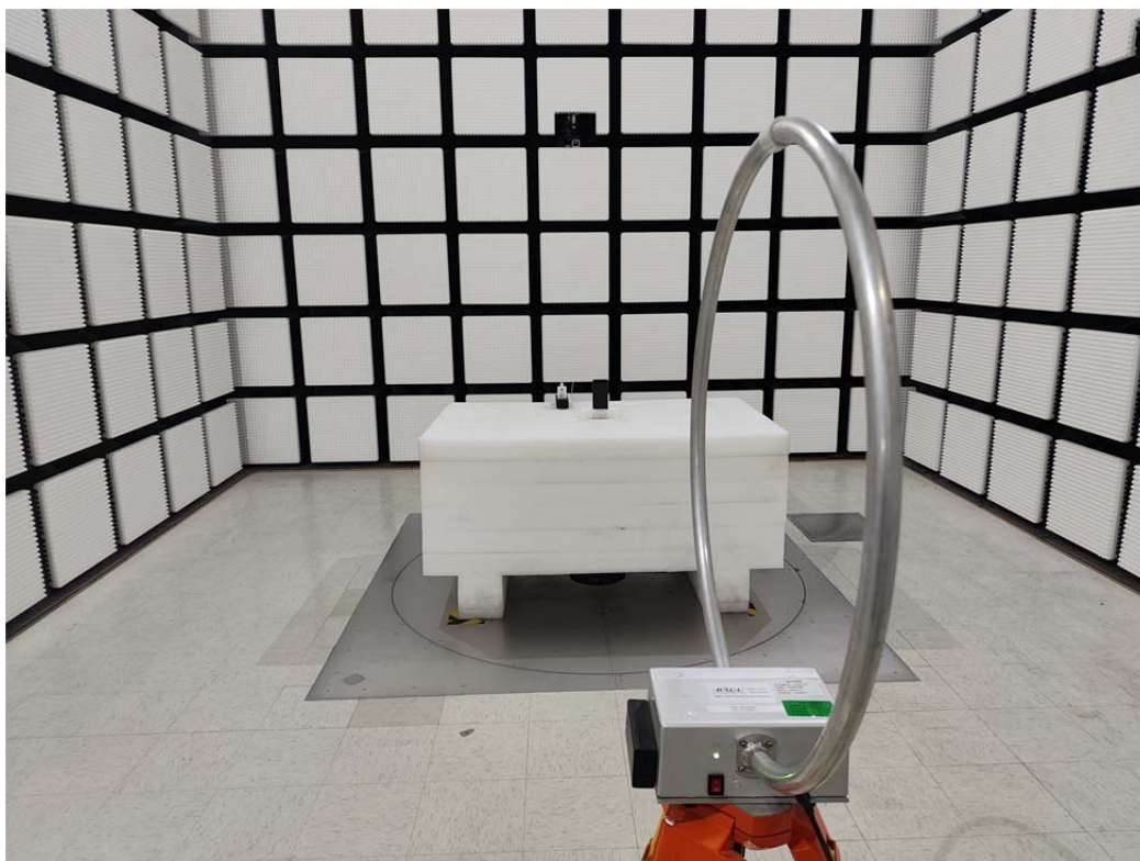
Radiated Emission 9 kHz-30 MHz Perpendicular View
