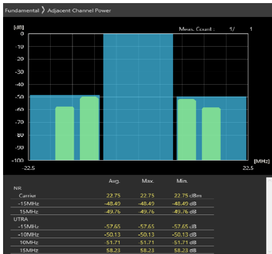
15MHz_30kHz_3557.5MHz-OFDM QPSK_RB36@0 -44.77,-46.03dB
