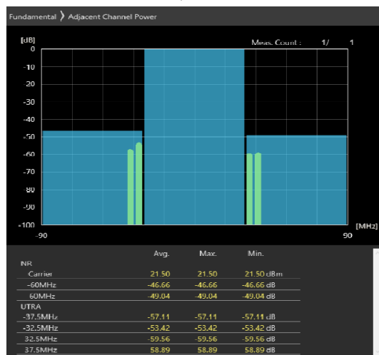
60MHz_30kHz_3670MHz-OFDM QPSK_RB162@0 -43.96,-42.82dB
