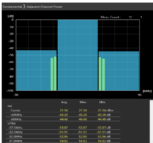
60MHz_30kHz_3580MHz-OFDM QPSK_RB81@40 -46.82,-48.22dB
