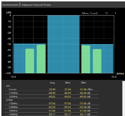
15MHz_30kHz_3557.5MHz-OFDM QPSK_RB36@0 -44.58,-45.82dB
