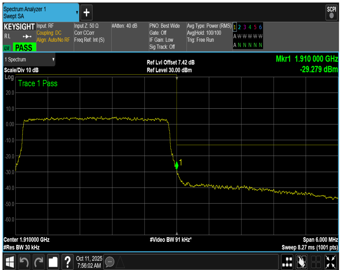
Band2 QAM16 BW=5MHz Channel=18625 RB Size=25 Position=#0
