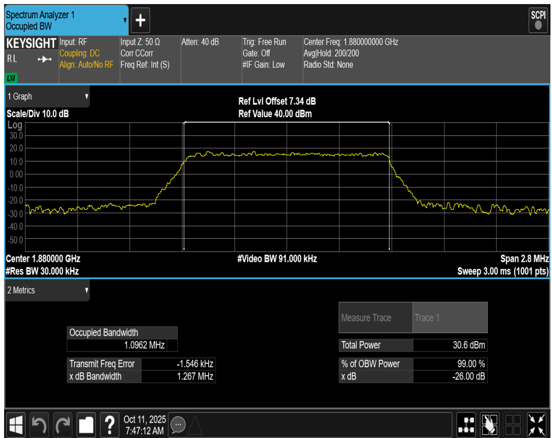
Band2 QAM16 BW=1.4MHz Channel=19193 RB Size=6 Position=#0
