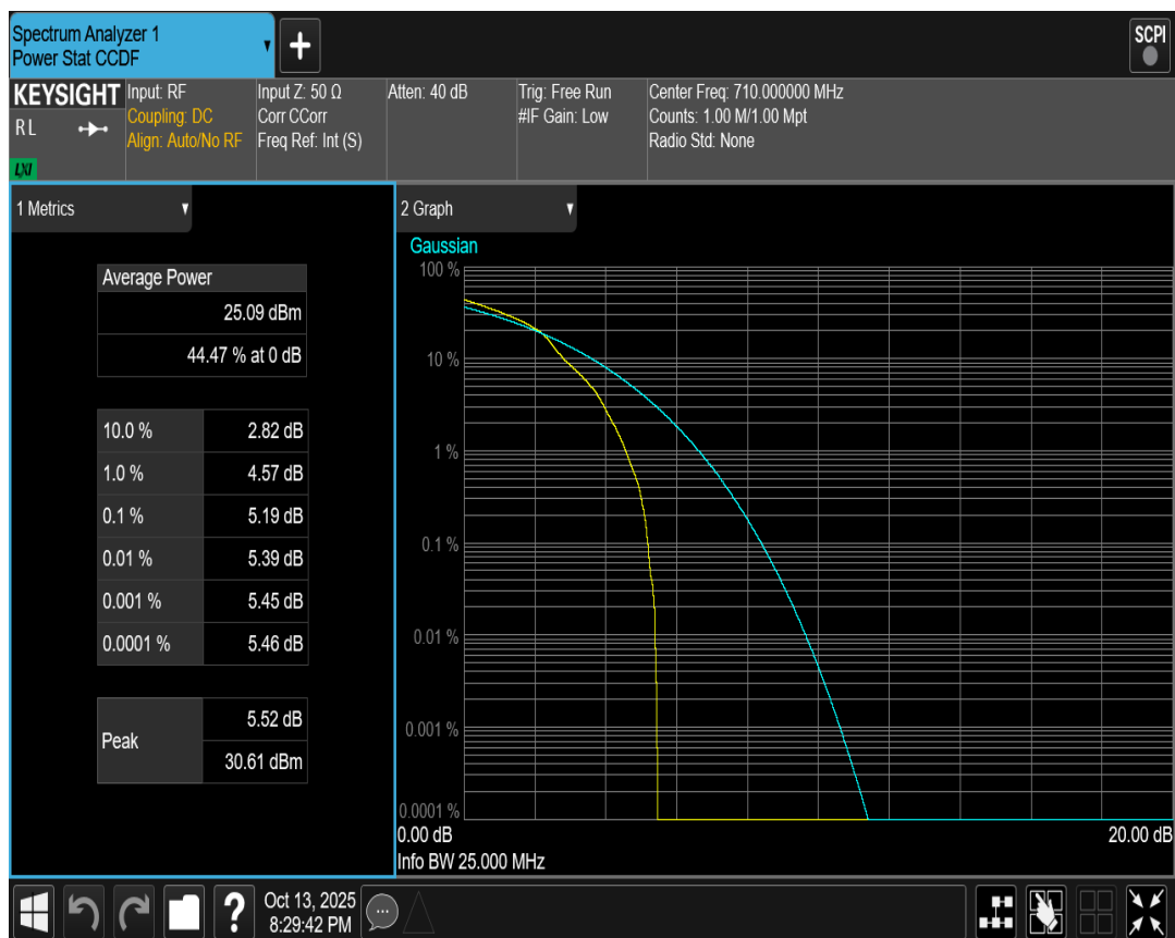
Band17 QPSK BW=10MHz Channel=23790 RB Size=1 Position=#0
