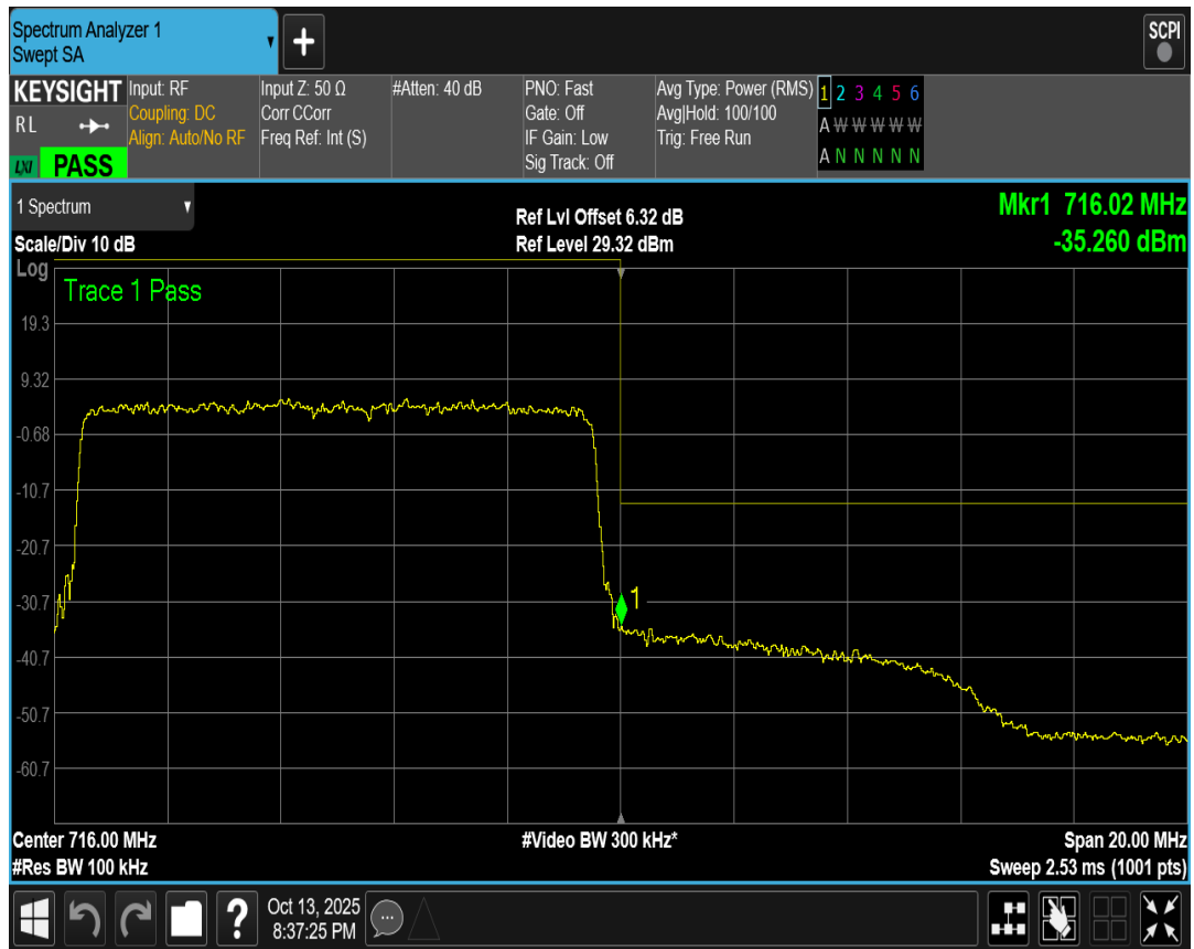
Band17 QPSK BW=5MHz Channel=23755 RB Size=25 Position=#0
