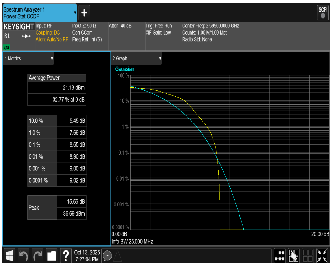
Band41(2535-2655) QAM16 BW=20MHz Channel=40640 RB Size=1 Position=#0
