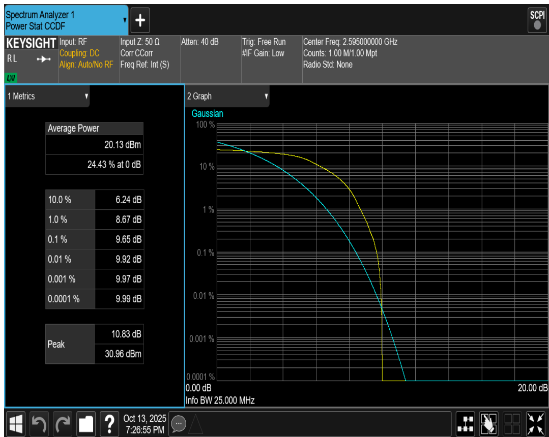
Band41(2535-2655) QPSK BW=15MHz Channel=40640 RB Size=1 Position=#0
