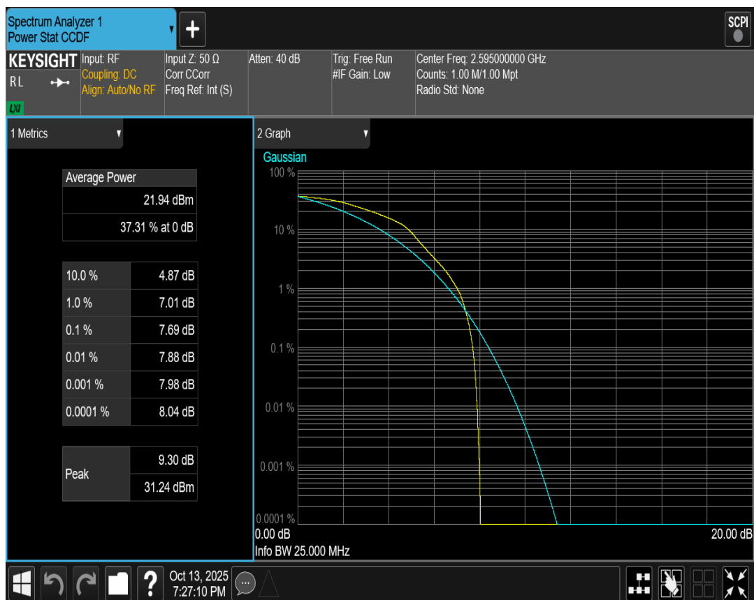
Band41(2535-2655) QAM16 BW=5MHz Channel=40640 RB Size=1 Position=#0
