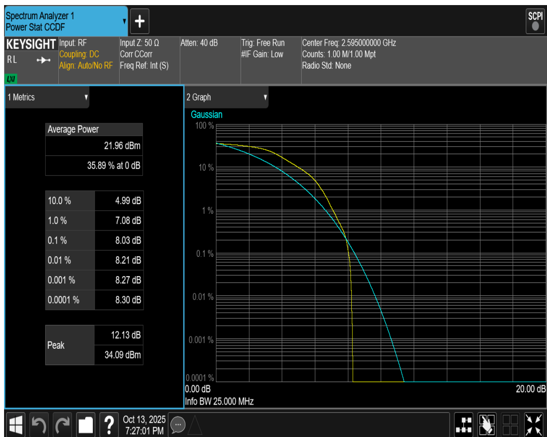
Band41(2535-2655) QPSK BW=20MHz Channel=40640 RB Size=1 Position=#0
