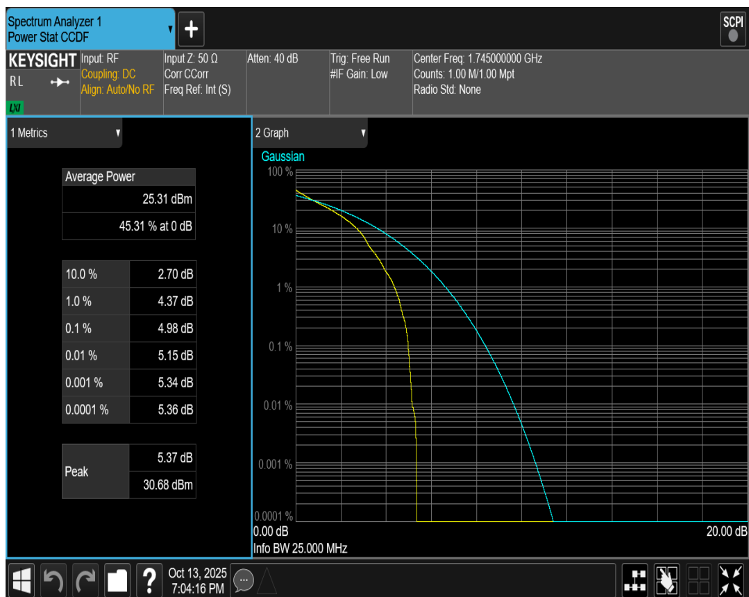
Band66 QPSK BW=5MHz Channel=132322 RB Size=1 Position=#0
