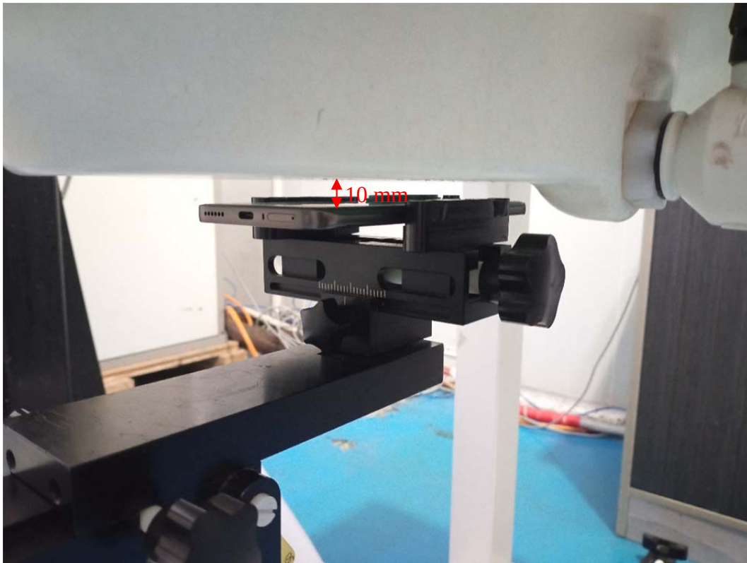
Body Back Setup Photo (10 mm)
