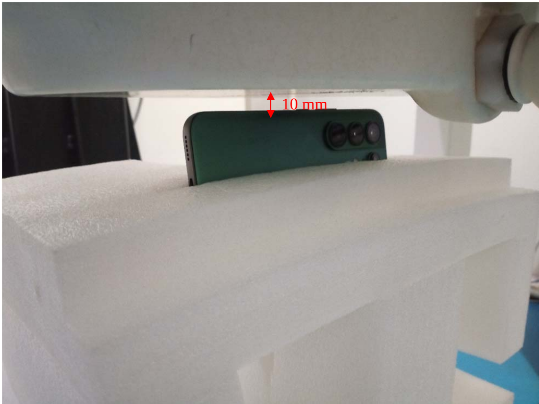
Body Right Setup Photo (10 mm)
