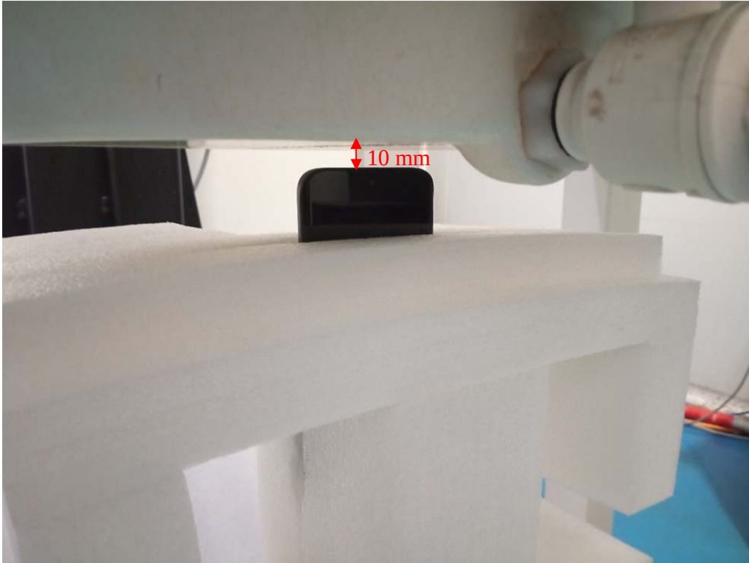
Body Bottom Setup Photo (10 mm)
