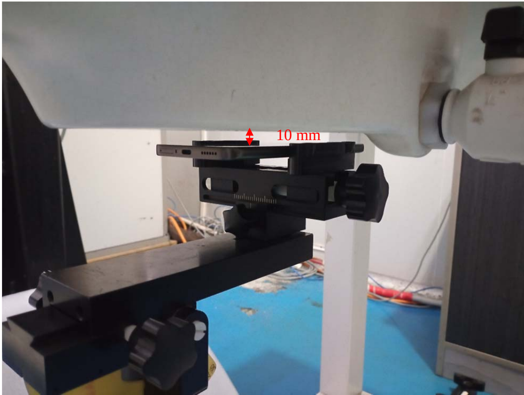
Body Back Setup Photo (10 mm)
