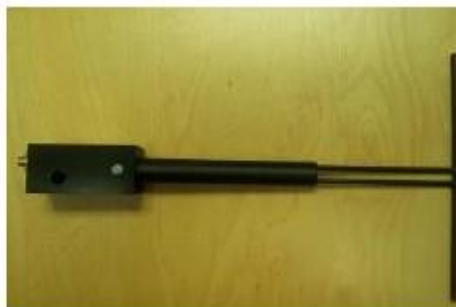
Figure 1 – MVG COMOSAR Validation Dipole
