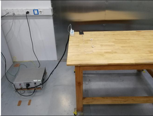
Conducted Emissions Test Setup Front View
