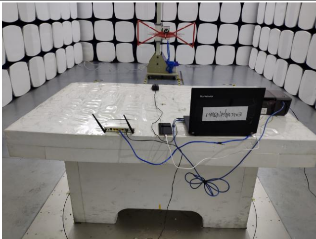
Radiated Emissions Test Setup Below 1GHz
