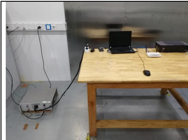
Conducted Emissions Test Setup – Front View
