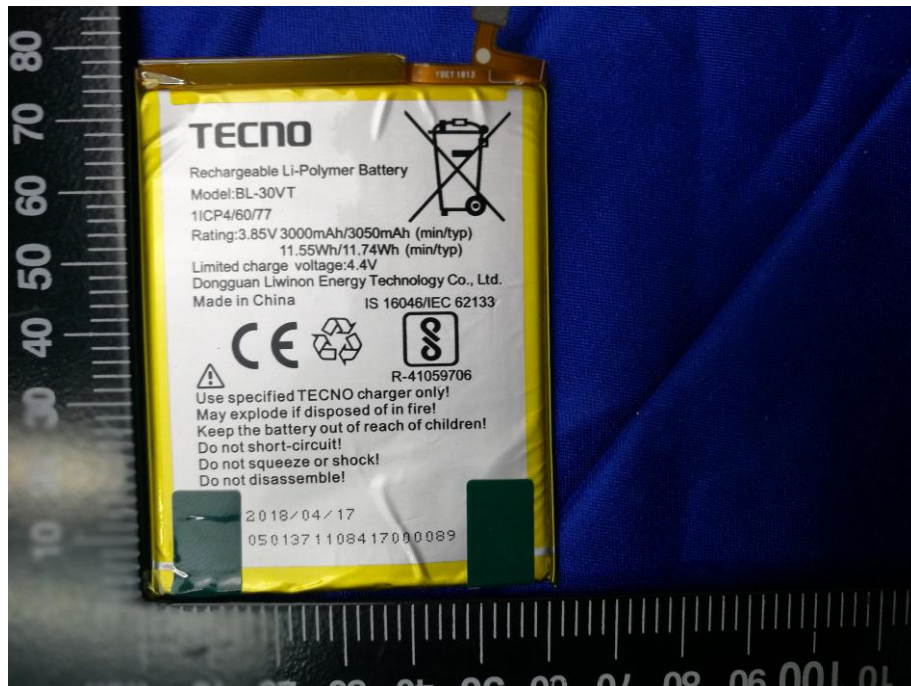
Battery - Front View
