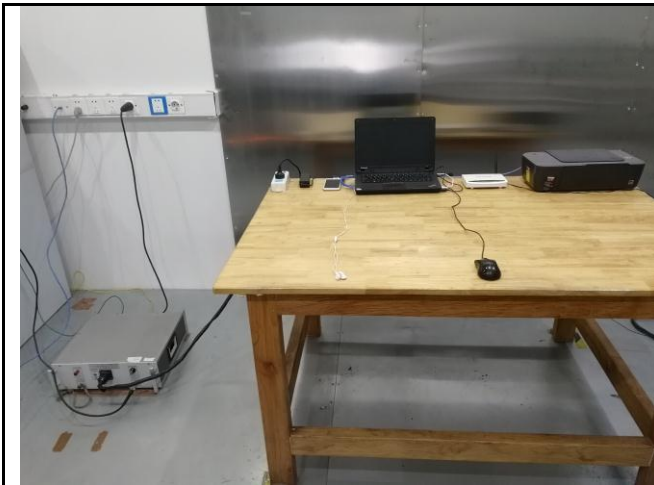
Conducted Emissions Test Setup – Front View
