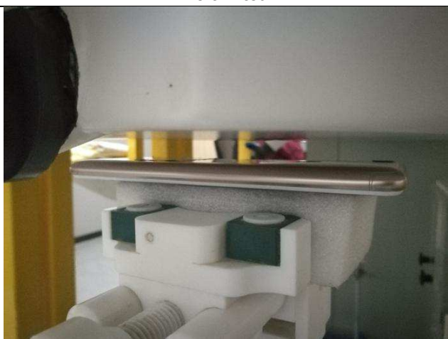
Rear Face of EUT with 1.0 cm Gap
