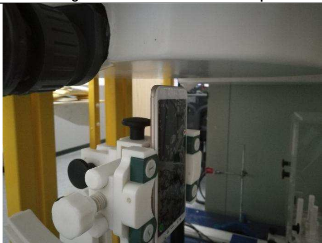
Bottom Side of EUT with 1.0 cm Gap
