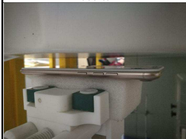
Front Face of EUT with 1.0 cm Gap
