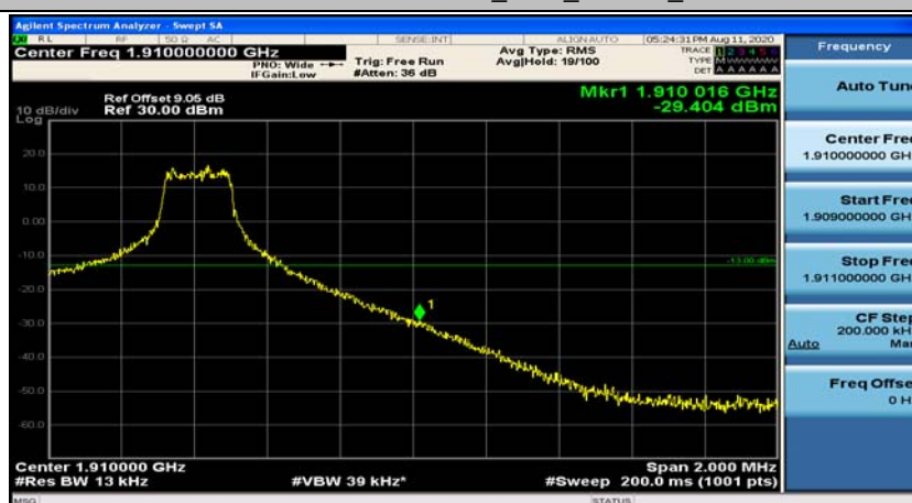
Channel Bandwidth: 10 MHz_HCH_16QAM_25RB#0
