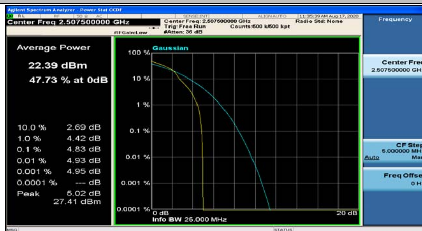
(Channel Bandwidth:15 MHz)_LCH_16QAM_37RB#0
