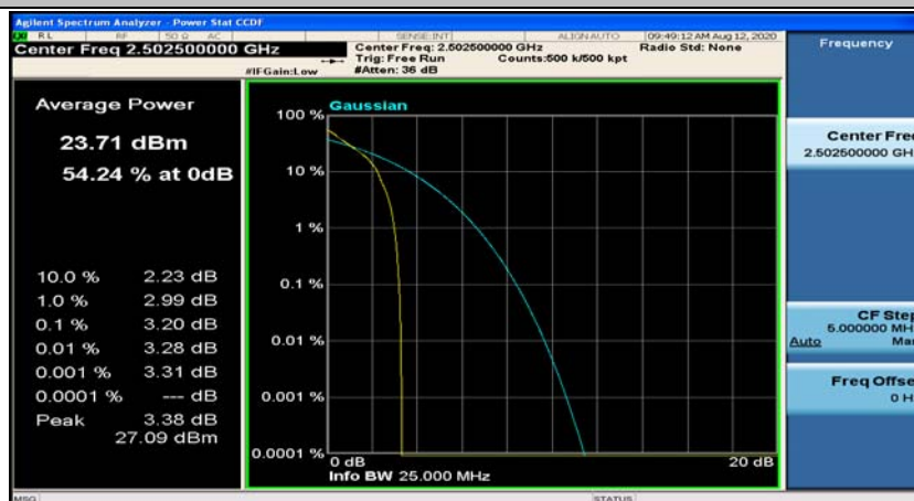
(Channel Bandwidth: 5 MHz)_LCH_QPSK_1RB#12
