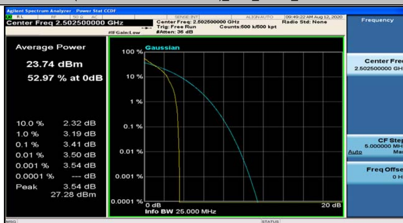
(Channel Bandwidth: 5 MHz)_LCH_QPSK_12RB#0
