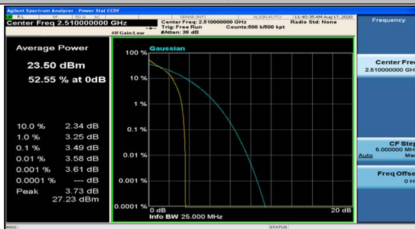
(Channel Bandwidth:20 MHz)_LCH_QPSK_1RB#99
