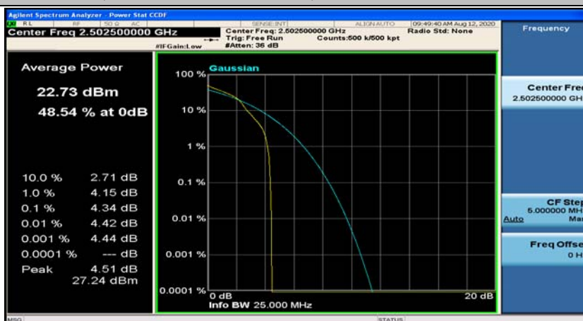
(Channel Bandwidth: 5 MHz)_LCH_16QAM_12RB#0
