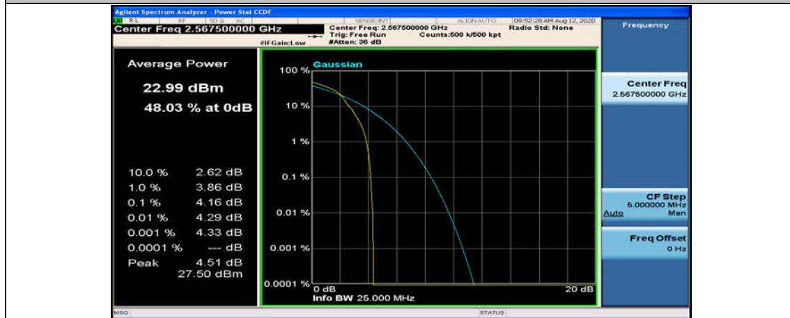
(Channel Bandwidth: 5 MHz)_HCH_16QAM_1RB#12
