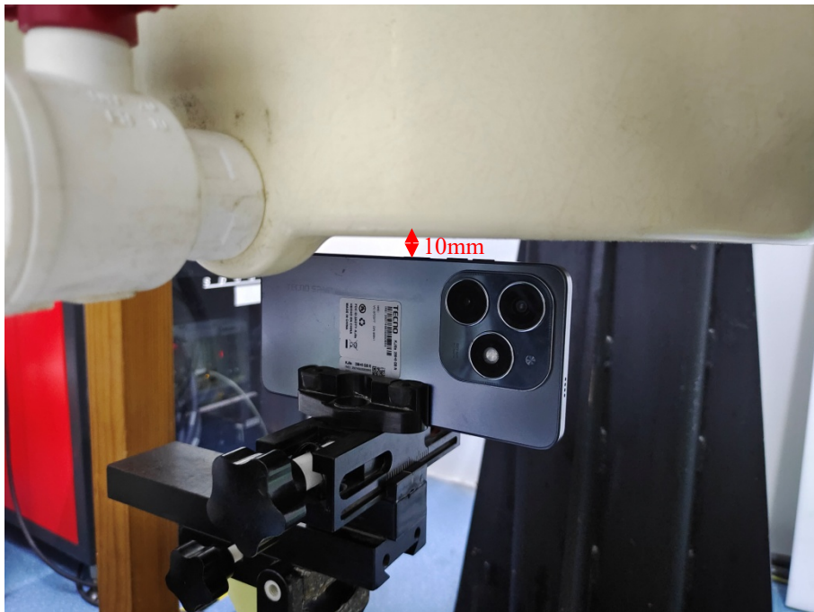
Body Right Setup Photo (10mm)
